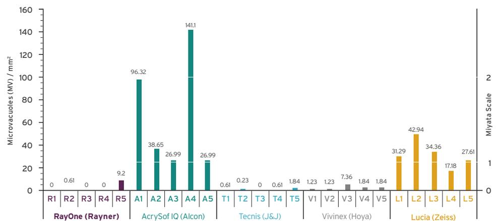
RayOne Hydrophobic reached 'significantly lower mean glistening numbers' compared to the AcrySof IQ (Alcon) and Lucia (Zeiss) IOLs ( $P < 0.05$ ).<sup>1</sup> A score below one on the clinical Miyata scale will not produce any significant visible glistenings on a slit lamp examination and is considered 'glistening-free'.
