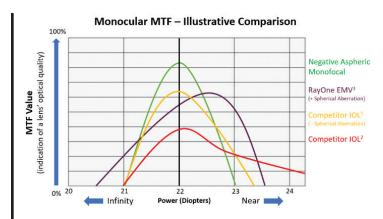
Figure 1. Illustrative comparison of modulation transfer function (MTF) curves. Compared to a negative aspheric monofocal, the RayOne EMV provides only slightly less power for distance, but much more useful vision at the intermediate range for activities like computer viewing.
