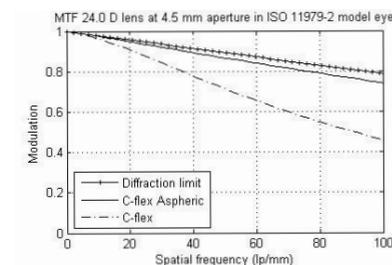
All IOL measurements were made at a 4.5 mm aperture and in accordance with the ISO 11979-2:2000 standard model eye.
